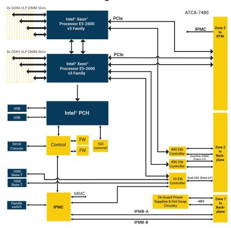
The Penguin Edge ATCA-7480 is fully backward compliant with RTMs available for the Penguin Edge ATCA Intel Architecture product portfolio. This easily allows extending the boards I/O and storage capabilities. The main I/O interconnect from the processor complex to the ATCA Zone 3 is based on PCIe supporting multiple I/O connections to meet high bandwidth requirements with up to Gen3.
